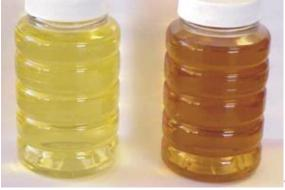
"After pulling a fluid sample from one of our hydraulic systems, we noticed that the hydraulic fluid had become darker. We were concerned, so we rushed the sample to the lab for analysis. The results of the fluid analysis appeared normal. The acid number, viscosity and oxidation by FTIR have all remained stable. A quick inspection of the hydraulic system revealed that the hydraulic valves have turned goldish in color. What should we do?"
